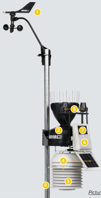
*Pictured: 6263 Wireless Vantage Pro2 Plus with 24-Hour Fan-Aspirated Radiation Shield*
