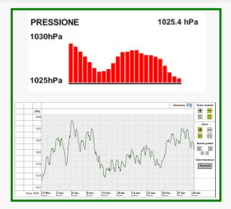
The atmospheric pressure measured may also be remotely compensated in order to match the pressure at ground level, as generally applied in meteorological applications.
