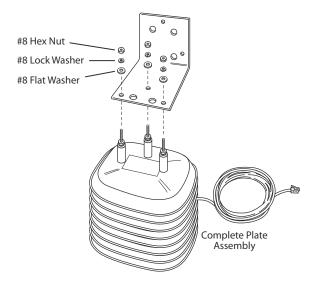
Hold the mounting bracket against the pipe and slide the ends of the two 1 1/2"
