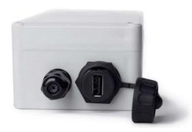
The data logger operates in a continuous mode. It does not just sample the measurements from time to time, but calculates ALL impulses generated by the sensors. The amount of impulses is recorded once a minute.
