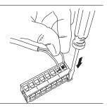
2. Connect soil moisture probes to the SOIL connectors.
