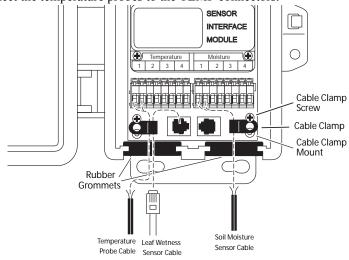
4. Secure all sensor cables through the provided cable clamps and then secure the mounts by driving a screw through the clamp into the cable clamp mounts located above the grommets.
